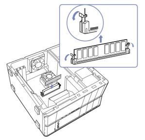
4 To insert a new memory module, remove it from its anti-static package, handling it only by the edges.
